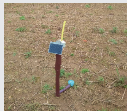
SOIL MOISTURE SENSOR IN THE FIELD AT THE ALLERTON PROJECT.
